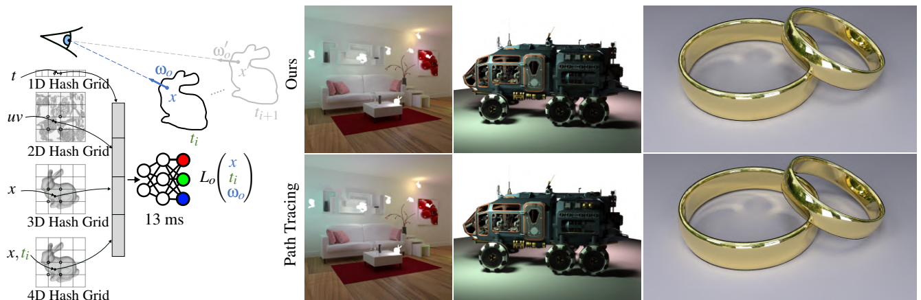
Figure 1: Our method uses a small neural network to explicitly represent a dynamic light field, acting as a radiance cache for spatio-temporal samples (x, \omega_o, t_i) . During inference, a simple visibility pass provides (x, \omega_o) samples at time t_i . Our novel combination of parameter encodings enables a small neural network to compute highly detailed radiance estimates in real-time. Due to the low computation cost of \sim 13 ms with all our encodings enabled, we can render a full neural light field of a dynamic scene with more than 60 frames per second in 1920 \times 1080 resolution. Additionally, our parameter encodings capture different scene dynamics within a compact memory footprint (40-80 MB). In the dynamic scenes above, our neural dynamic light field representation is \geq 20 times faster than previous works [HCZ21, DPD22].
